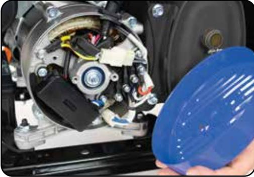
The carbon brushes in conjunction with the AVR regulates power from the generator. If the generator is overheated or overloaded, the AVR may be damaged and require replacement.
