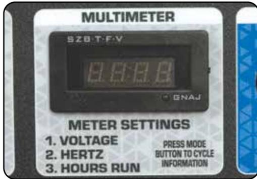
When the generator is started, the display will read the current voltage. Press the MODE button to cycle through the multimeter functions.
